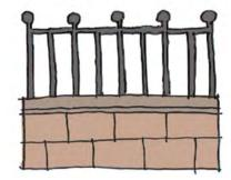
Stone wall with coping and metal railings above. Up to 1m in height when used at front. Up to 2m to side and rear (wall max 1m) with piers at regular intervals.
