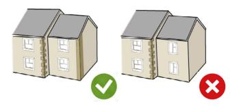
Observe existing design details that are used at the junction between one building material and another.
