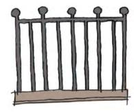
Metal railings on stone plinth up to 1m high when used at front. Up to 2m to side and rear.
